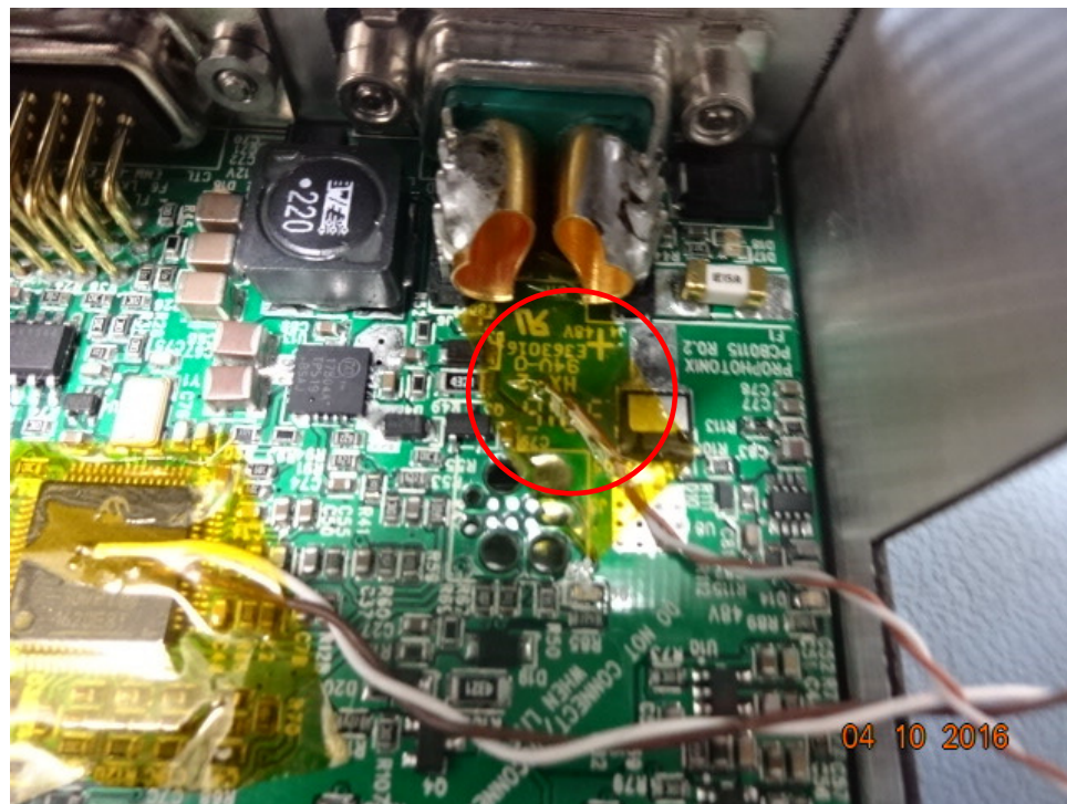
Figure 14: PCBA thermocouple location
