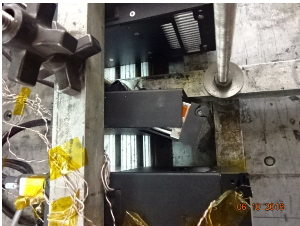
Figure 20: Front Face off on FX1 395 unit loose screws and damaged cover
