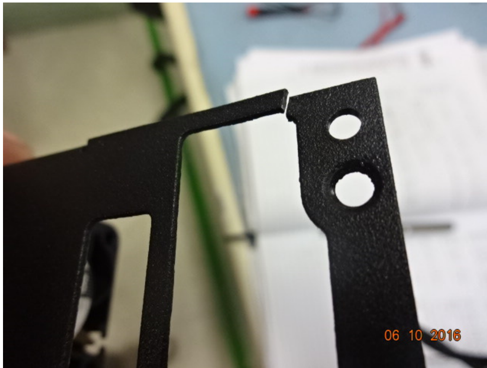
Figure 19: Cover Damage on unit following vibration testing
