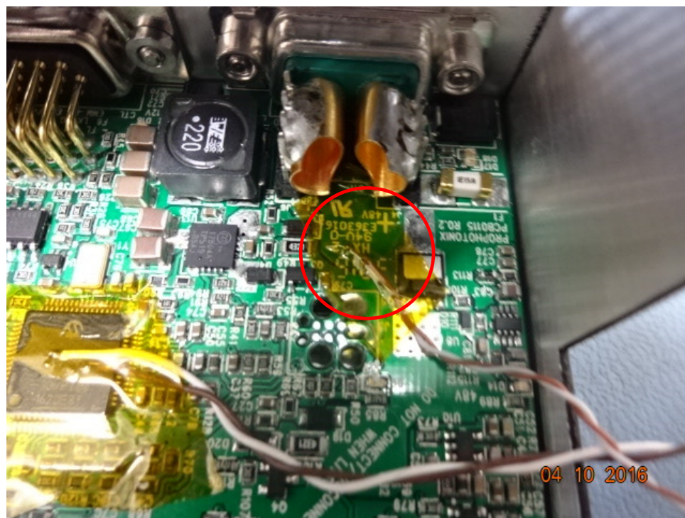
Figure 14: PCBA thermocouple location
