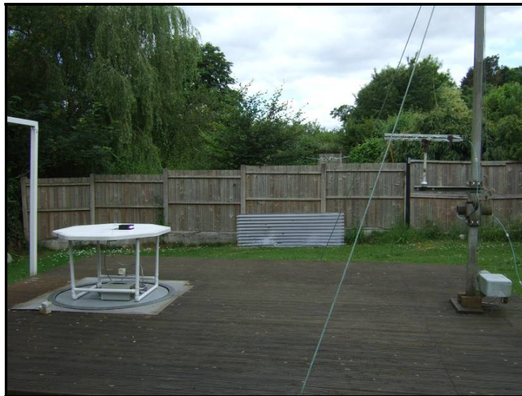
Photo 4 UHF setup of EUT with antenna in horizontal position.
