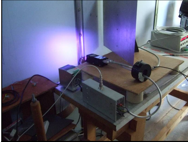
Photo 7 EUT setup for direct injection on DC power line.
