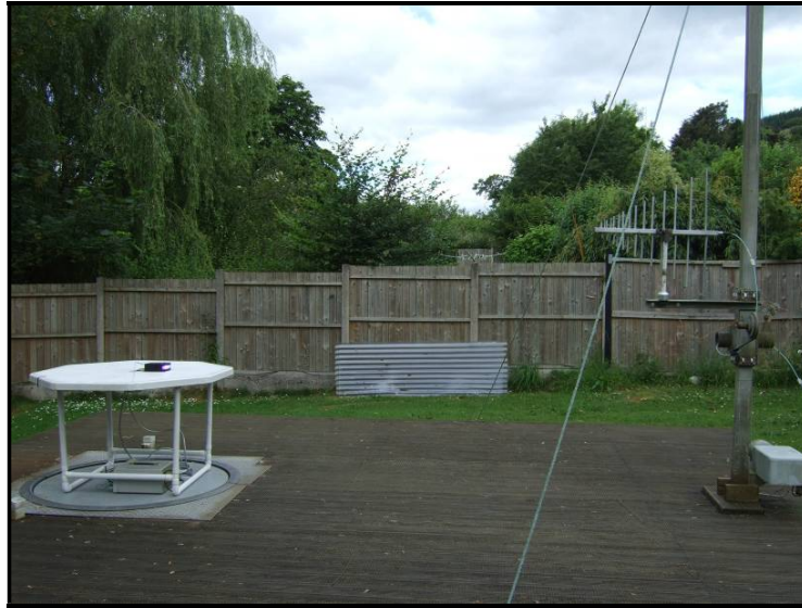
Photo 3 UHF setup of EUT with antenna in vertical position.
