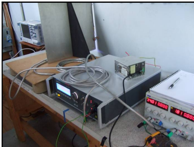
Photo 6 Layout for EFT tests with direct coupling on DC power lines.
